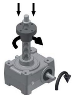
Righthanded worm screw and left-handed lead screw.
